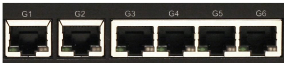
Figure 1.3. The E80 Ethernet Interface Ports
