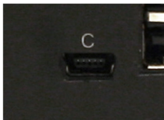
Figure 3.1. The E80 Mini-USB Local Console Port
